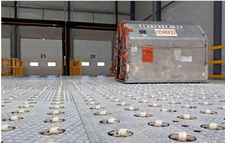
Cargo Castors are essential components used in ULD handling environments at airports worldwide. You can find our silent and maintenance free products in logistic cargo centers. But also on Ground Support Equipment (GSE) like dollies and loaders on the ramp our products are used intensively.
